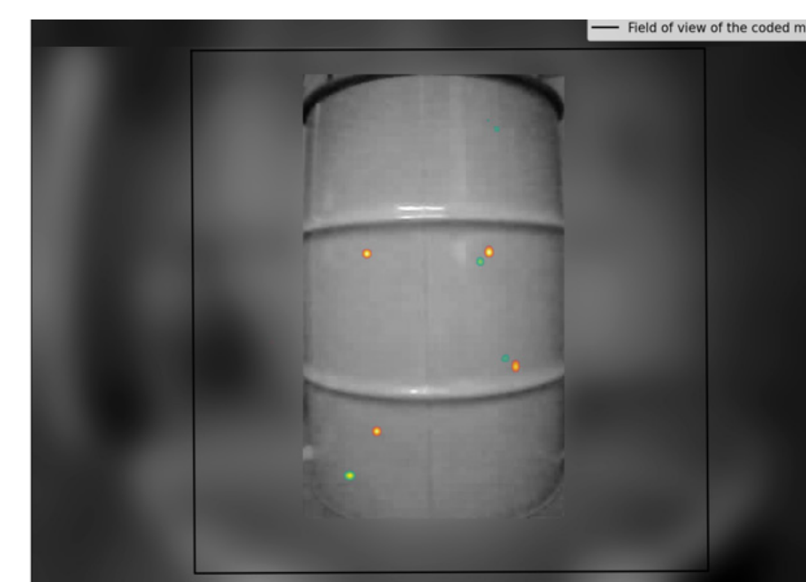
Green : 152 Eu sources, 10 MBq per source Orange : 241 Am sources, 3,6 MBq per sources
