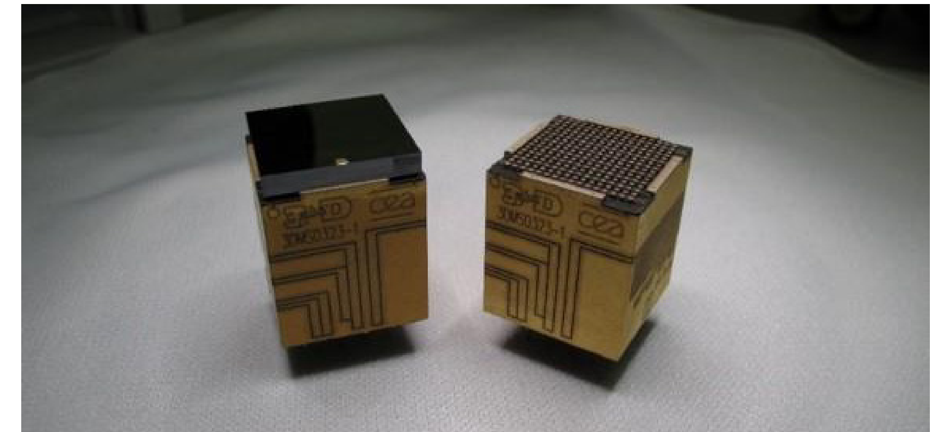
The Caliste-O 3D module is the latest development of the Caliste technology which started in 2006. It is made of 8 IDeF-X ASICs moulded with the 3D PLUS technology to form a 3D electronic part, on which a CdTe cristal of 1.4 x 1.4 cm 2 and 2 mm thick is mounted.
