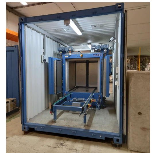
Fig. Mirion Technologies RTM644Inc large clearance monitor
